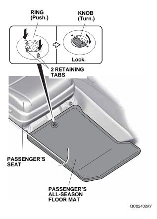
4. Install the rings in the left and right rear all-season floor mats over the anchors. Push the rings into the anchors to secure the retaining tabs, then turn the knobs 90° to secure the mats to the floor.
